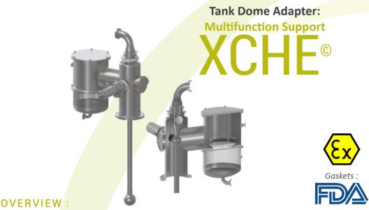
The XCHE is a device placed on the dome of a tank. At a single point, it can be fitted with equipment for pressure (SHP safety valve) and vacuum protection (BOG or HSV-A vacuum break valves depending on diameters), for washing the tank, the XCHE and all its components, and for pressurising and recovering fermentation gases (CHE washing check valve). The XCHE is also equipped with additional taps, for stainless steel rupture disc and/or for pressure sensor.
